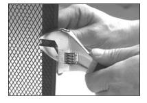
**6e.** Proper installation of the latch assembly.
